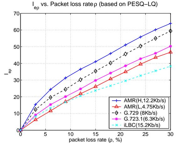
Fig. 4.  $I_{e\rho}$  vs. packet loss rate  $\rho$
